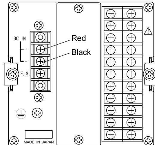
Connect the positive (+) side of the power source to the red screw side of the terminal block on the back of the F370, and its negative (-) side to the black screw side.
