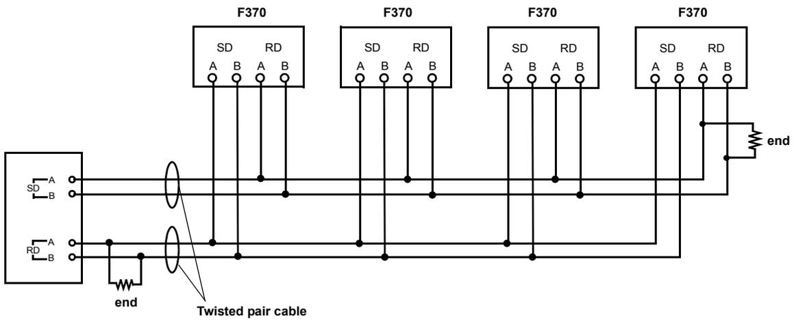
Use a twisted pair cable for connection. (The noise margin will increase.) However, a twin cable is sufficient for short-distance connection. Couple a terminal resistor of 100 - 200  $\Omega$  to the receiving end.
