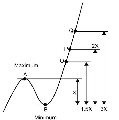
When difference  $X$  between detected relative maximum value A and relative minimum value B exceeds the predetermined detection levels (1.5, 2 and 3 times), A is displayed in the maximum value hold mode at respective points O, P and Q and the value is held.
