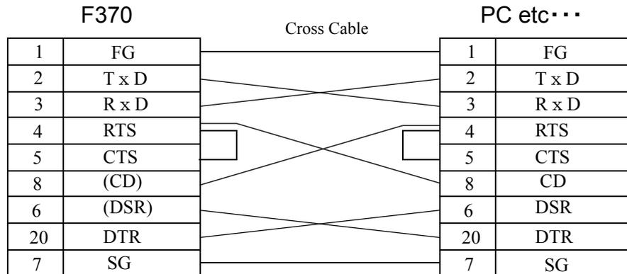
\* This connection diagram shows an example of connecting a DTE (data terminal equipment) personal computer.
