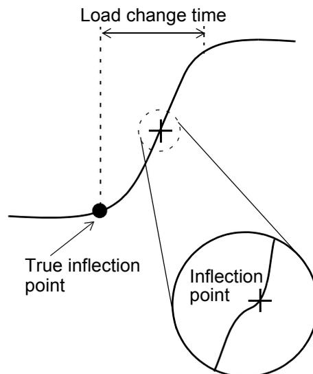
If the detection interval A and B are set too short, fine load changes may be detected as shown in the illustration on the left-hand side, so that a correct value cannot be held.
