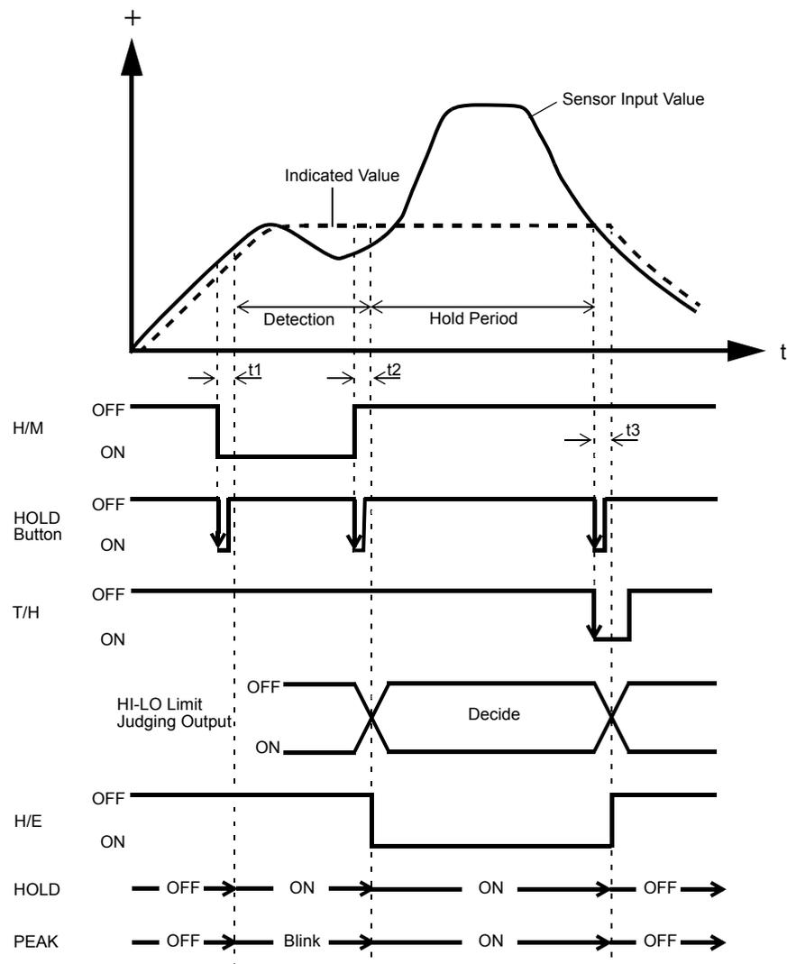
$t_1$  : A delay time between the instant when the H/M signal is inputted and the instant when the value to be held is detected
