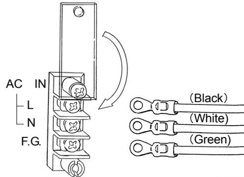
Connect AC power code attached to the terminal.
