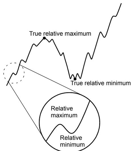
If the minimum count is too small, when the waveform includes noise as shown on the left-hand side, the noise is regarded as the relative maximum value or relative minimum value and a correct value may not be held. In such a case, set the minimum count somewhat large.
