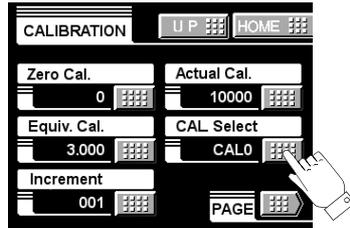
4) Select the calibration value from 0 - 3 and determine with the OK button.
