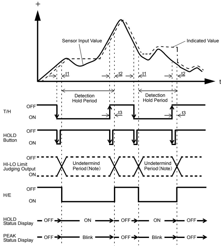
Note: During the undetermined period, the judging output varies with fluctuations in the input waveform. However, the H/E output remains on during the undetermined period. Read the judging result when the indicated value becomes stable (immediately before the T/H signal rises).
