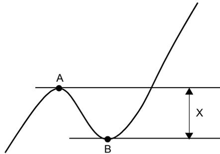
First, when difference  $X$  between point A and point B is larger than the minimum count, point A is judged to be the relative maximum value and point B is judged to be the relative minimum value.
