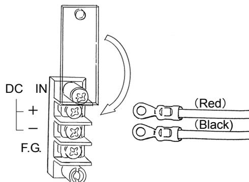
Connect the positive (+) side of the power source to the red screw side of the terminal block on the back of the F370, and its negative (-) side to the black screw side. The input voltage is 12V - 24V DC.
