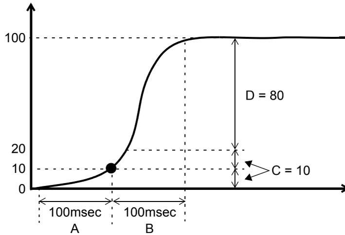
① Set the load change time (between the inflection point and when the change stops) to interval B.
