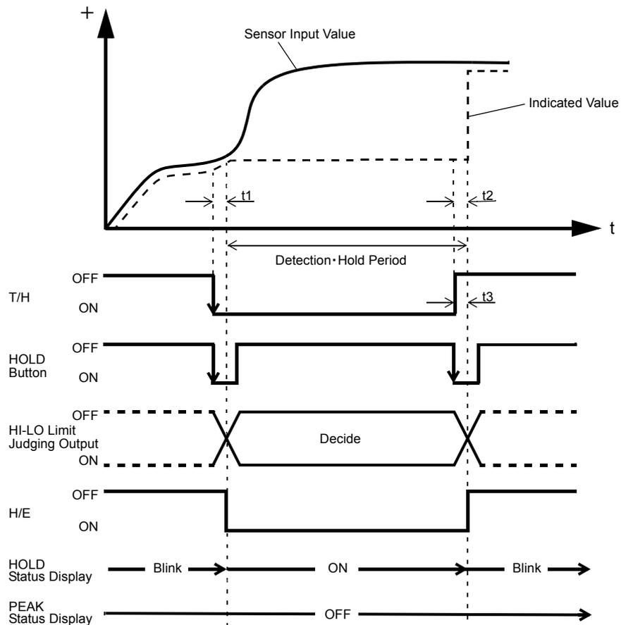
$t_1$  : A delay time between the instant when the T/H signal is inputted and the instant when the indicated value is held
