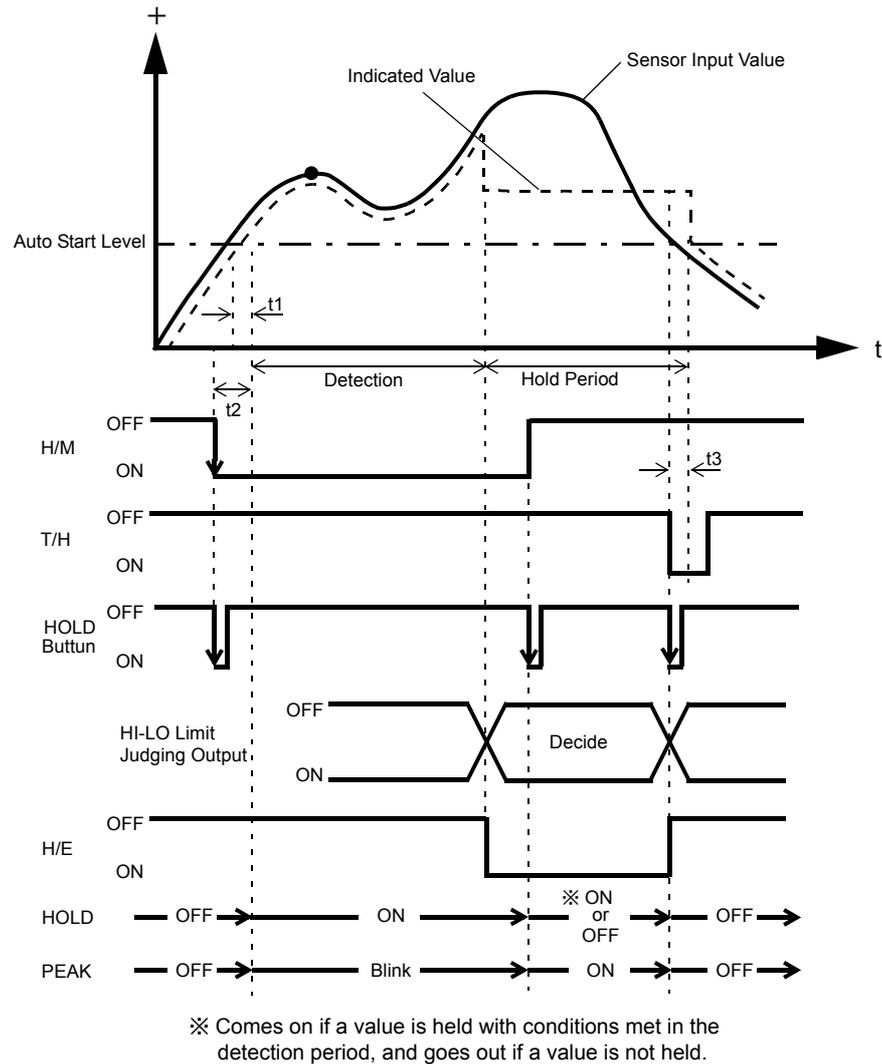
t1 : A delay time between the instant when the indicated value exceeds the auto start level and the instant when the value to be held is detected
