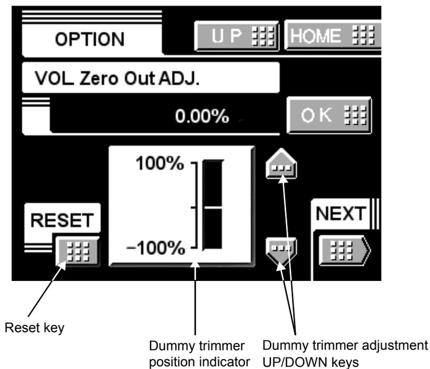
\*Pressing the dummy trimmer UP/DOWN keys continuously performs continuous operation.
