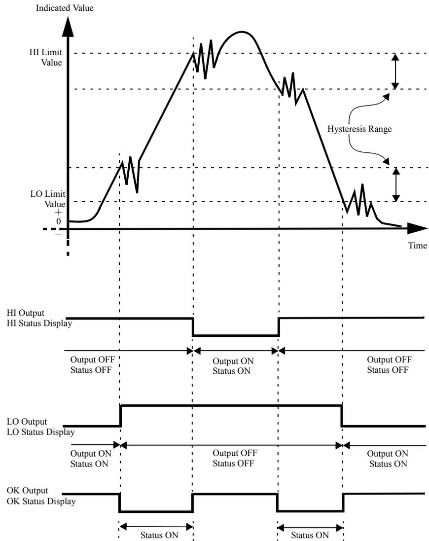
( Exsample : HI Output and LO Output and OK Output )
