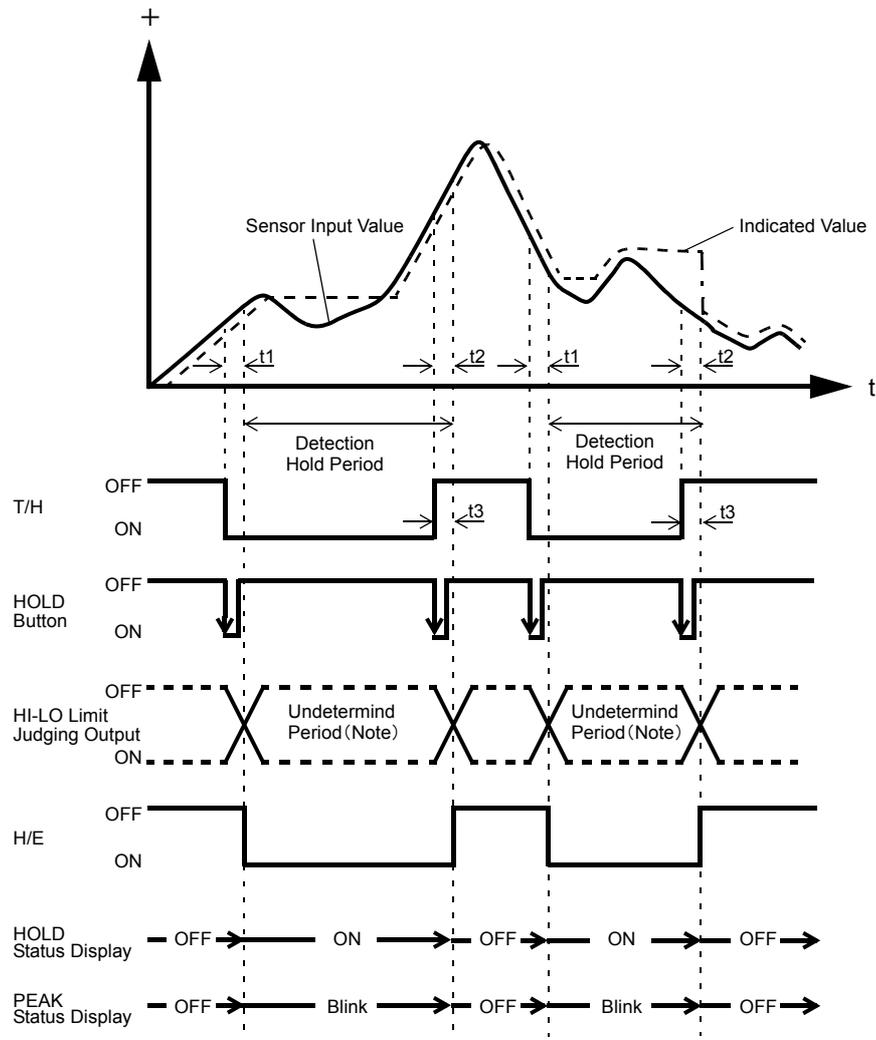
Note: During the undetermined period, the judging output varies with fluctuations in the input waveform. However, the H/E output remains on during the undetermined period. Read the judging result when the indicated value becomes stable (immediately before the T/H signal rises).
