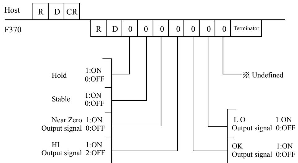
※ The hold bit is operated at the same timing as the H/E signal.
