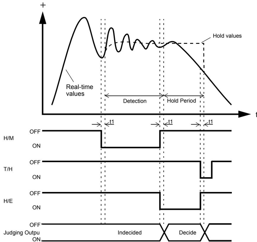
t1 : A delay time between the instant when the T/H or H/M signal is inputted and the instant when operation is performed.
