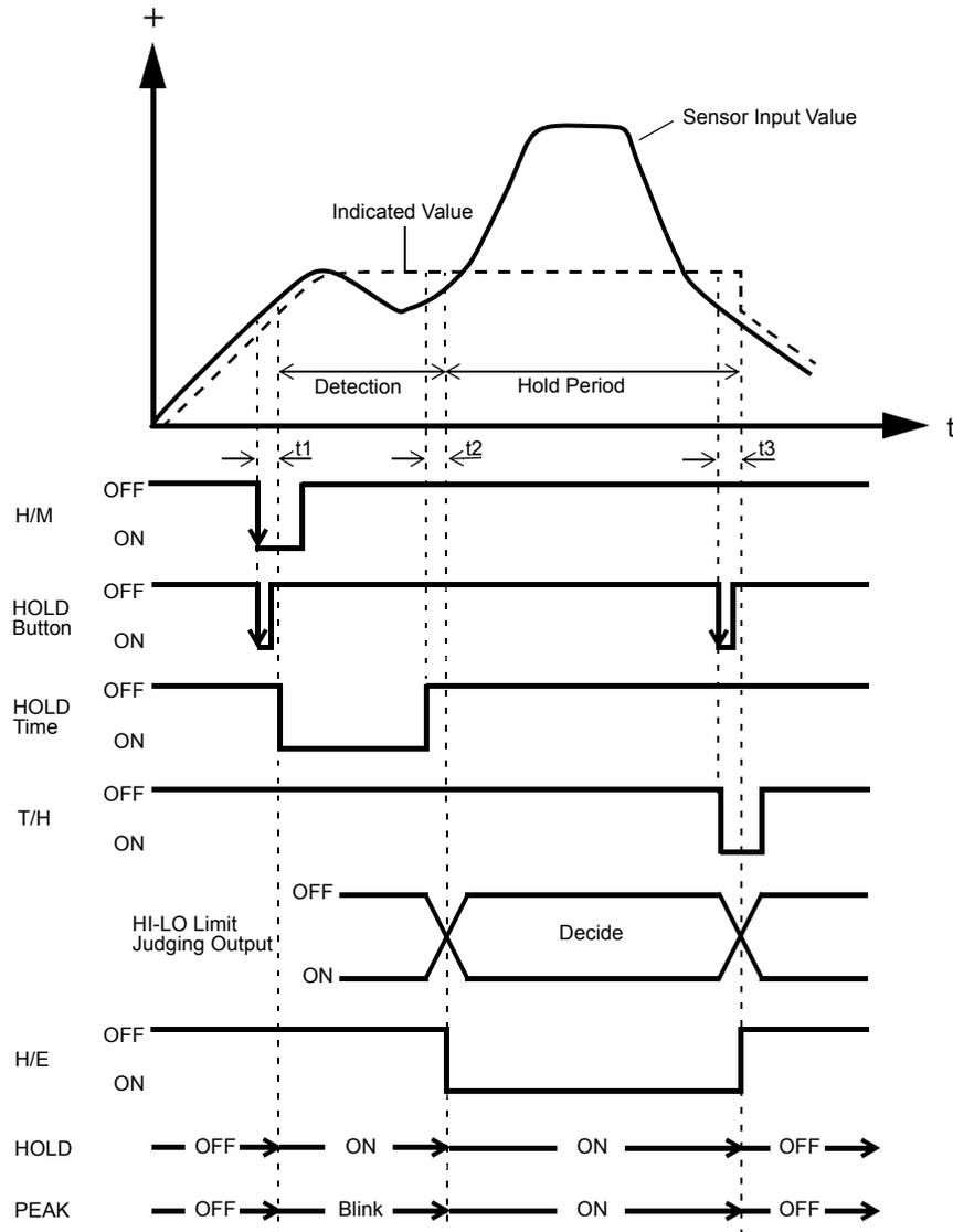
t1 : A delay time between the instant when the H/M signal is inputted and the instant when the value to be held is detected
